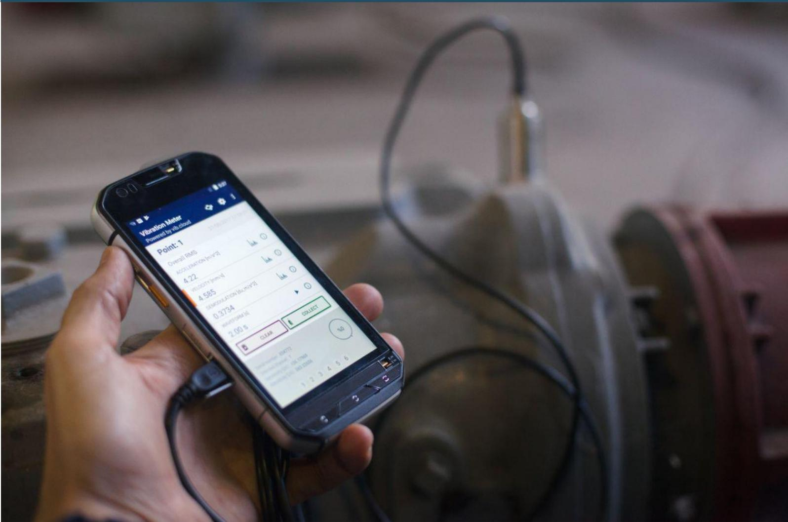
Mobile application for vibration measurement and on-the-spot diagnosis. Works with Digiducer vibration sensor or use your own ICP sensor utilising new digital ICP signal conditioner
